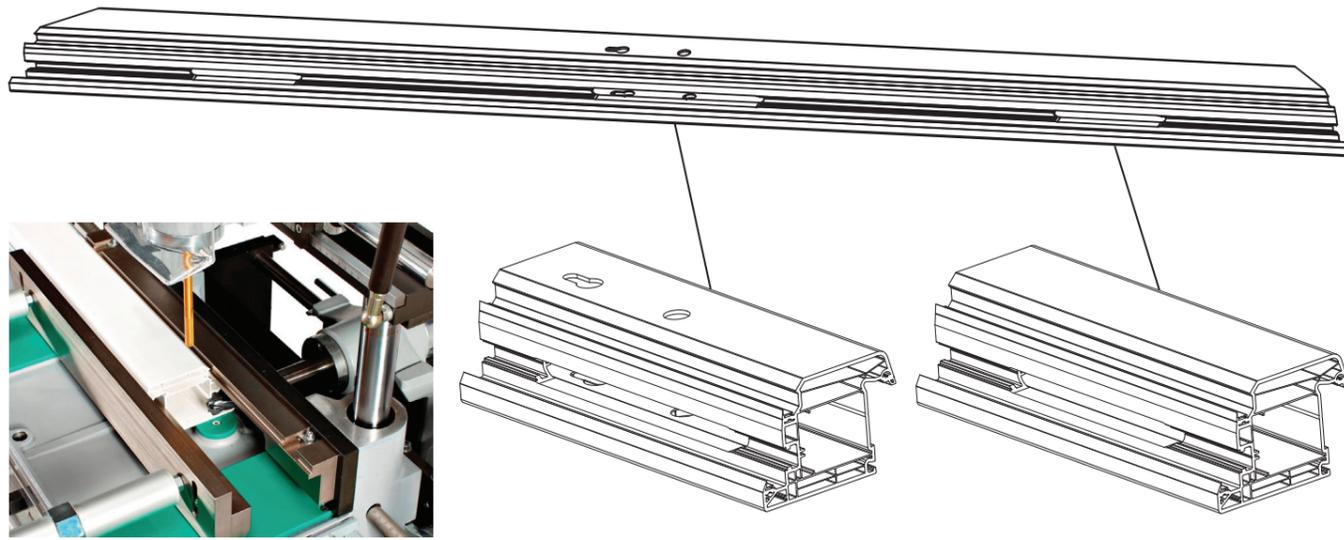
6+6 foldaway stops on the lateral supports in 3 available lengths: 1-2-2,5m.
