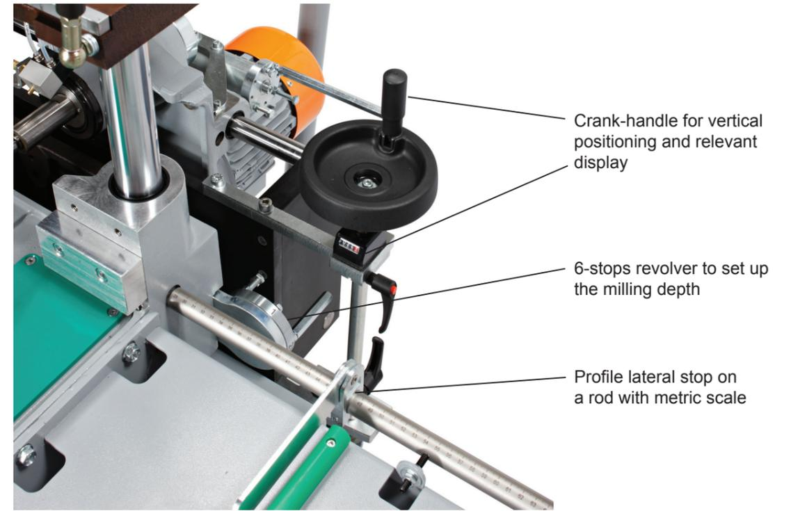
The rear unit regulations are made from the operator post.
