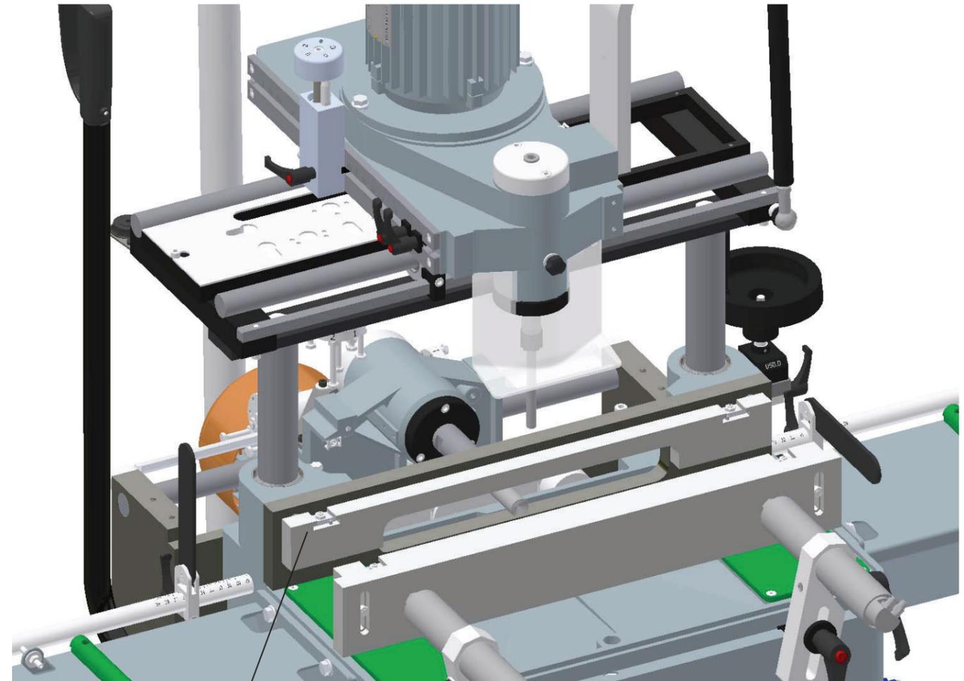
The main feature of the clamping system is represented by its customized counter shapes that firmly secure the profile to the working table without any vibrations and deformation. The counter shape change is extremely fast thanks to the easy reverse system.
