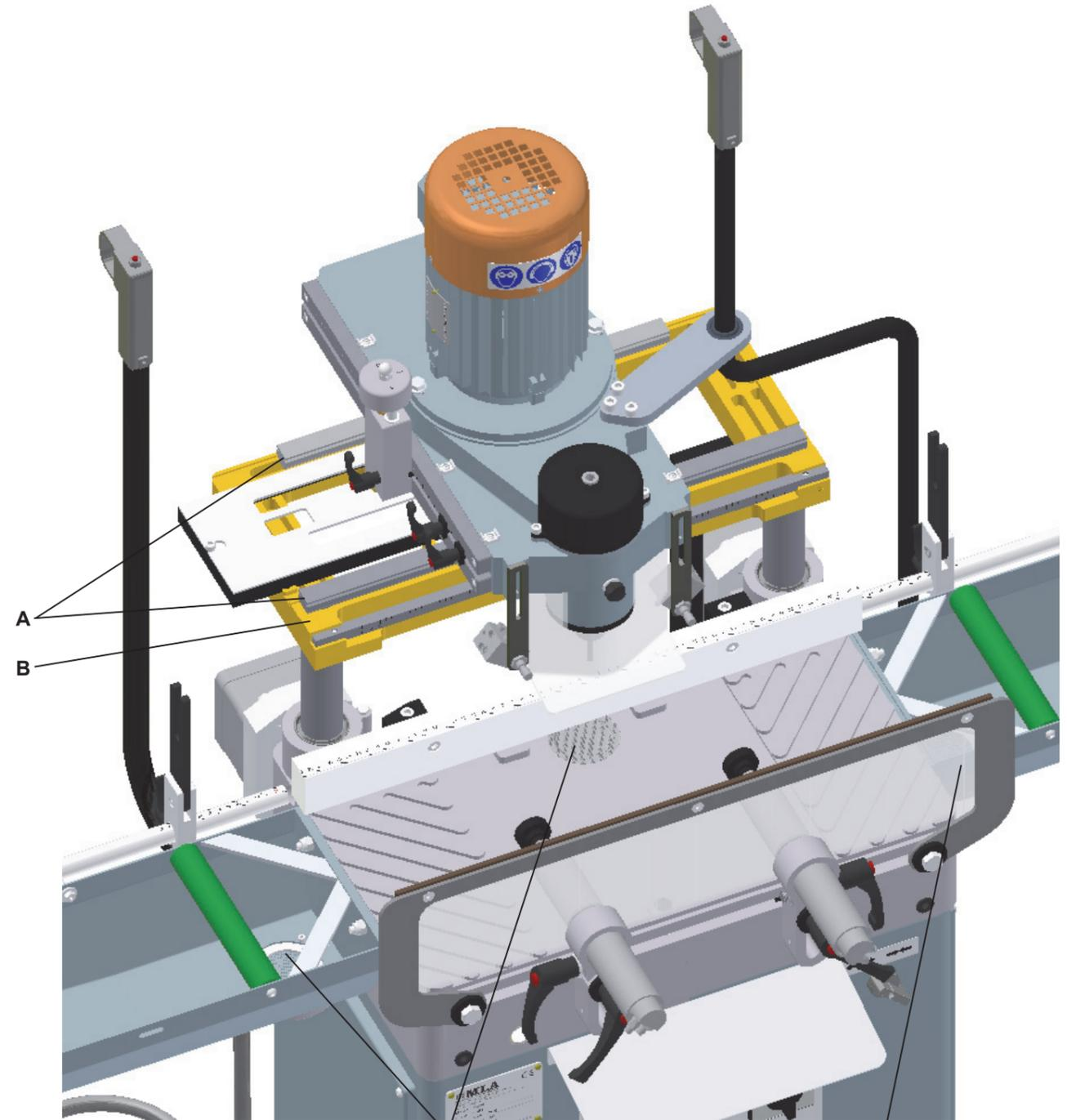
Linear rail guides (A, axis x and y) are fixed on a strong cast iron support (B), which enables the operator to work in a very stable way and without vibrations.
