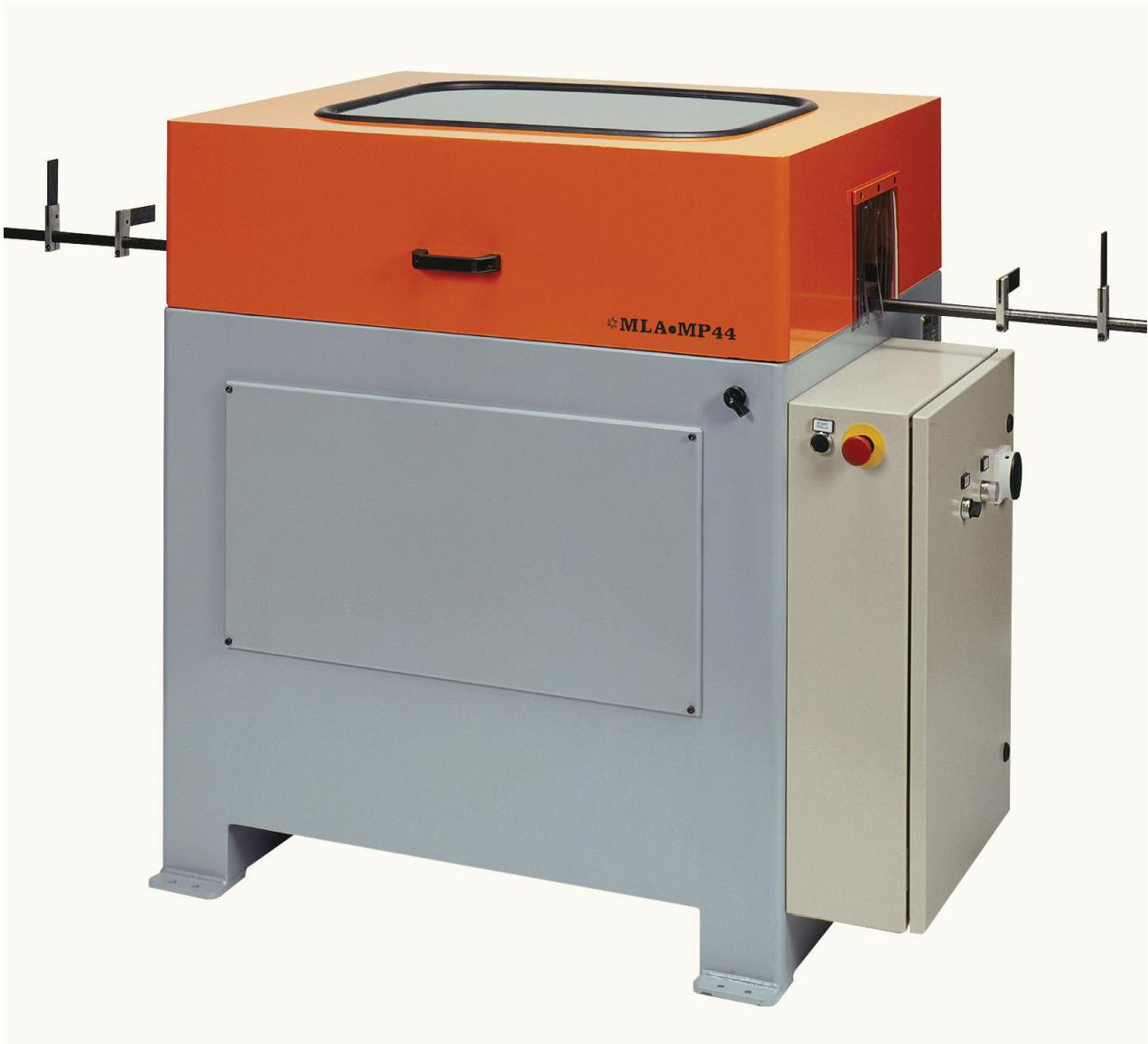
MP44 carries out the slots to insert the ventilation grids with a high productivity automatic cycle thanks to two opposing pairs of motors.
